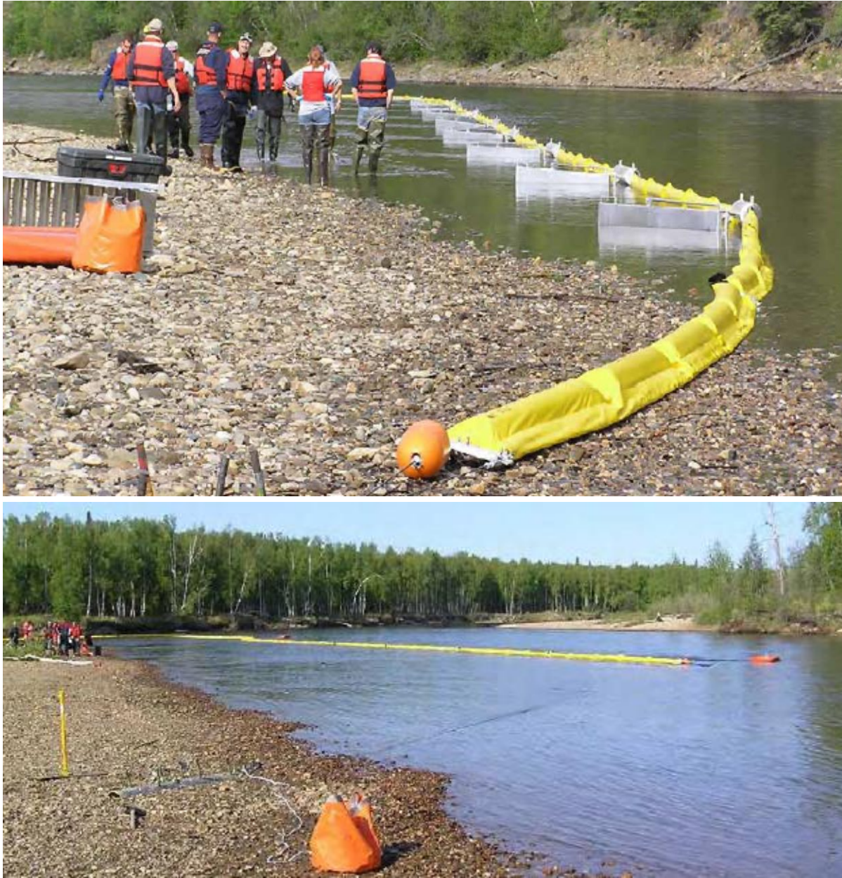
Figure 14—Boom Vane. Top: Boom Deployed with Deflectors/Rudders. Note the Boom Vane on the Shoreline. Bottom: Leading Edge Controlled by a Mooring Line Secured to Anchor Plate
