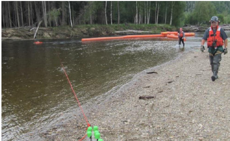
Figure 16—Current Buster 2 Deployed with Boom Vane in a River
