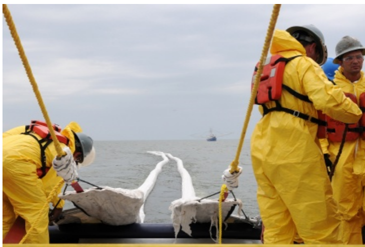
Figure 5—Fire Boom Being Deployed from Vessel During Training (USCG, 2010a)
