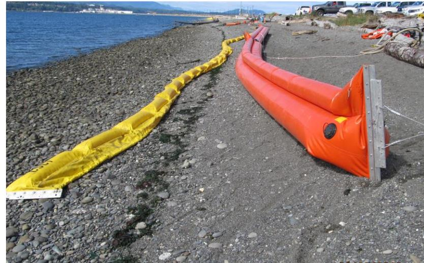
Conventional solid floatation boom and water-ballasted (“shore-seal”) boom deployed at the high tide water level during an exercise (Port Angeles, WA).
