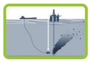
SUBSEA DISPERSANT APPLICATION MINIMIZES DIRECT HUMAN CONTACT WITH DISPERSANTS, OIL, AND VOLATILE FUMES
